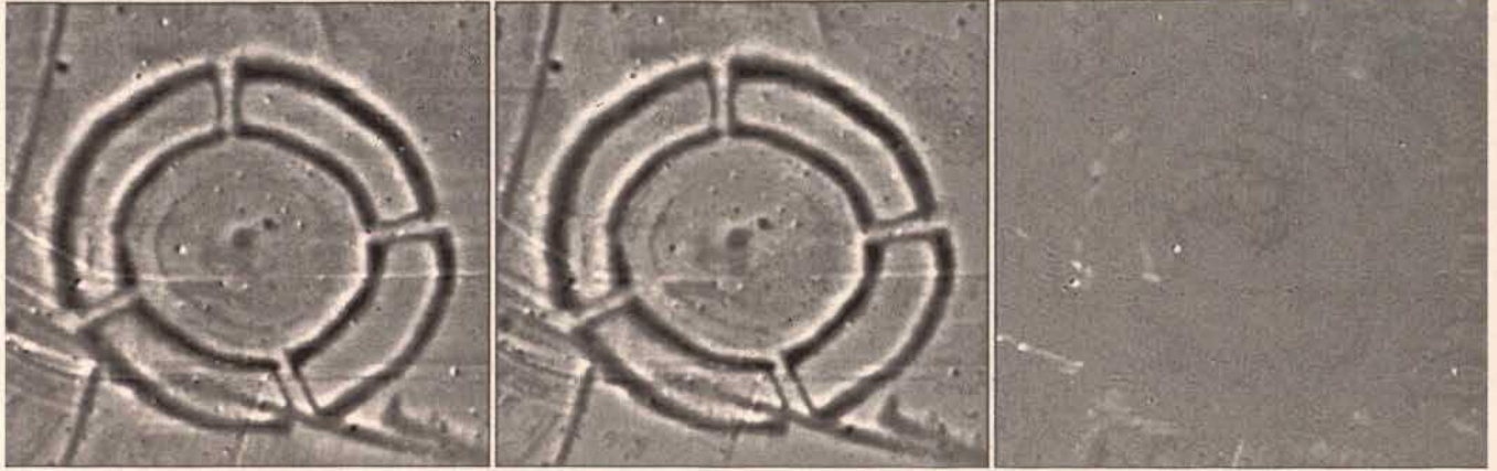
Fig. 1. The comparison of the measured and reconstructed anomalies shows the equally good reconstruction of all parts of the monument; caesium gradiometer 0.5 m – 2.0 m; raster 0.5 m x 0.25 m; area 110 x 105 m; visualised anomalous range [-6,15] nT
