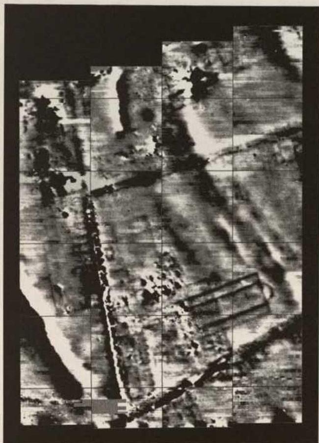
Fig. 6. Ostia Antica 1996 Magnetogram (detail with the basilica of Constantinus I.) in greyscale, dynamics -50.00/+50.00 nT in 256 greyscale (white/black), sensitivity \pm 10 pT, raster after resampling 0.5/0.25 m, 1 Hz bandpass-filtering, reduction on 40 m line means, 40 m grid, Mag Nr. OS96-A
