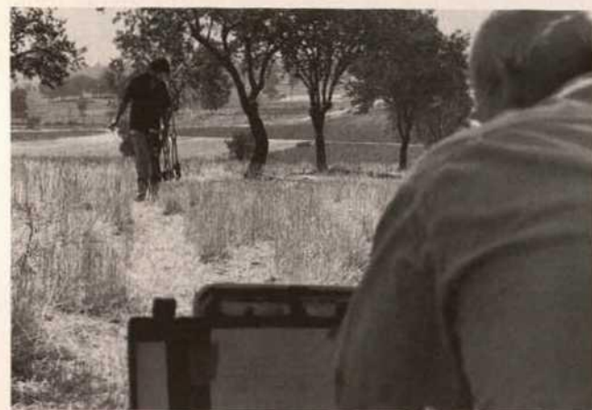
Fig. 3. Troy 1992. Magnetic prospecting in the lower city of Troy in 1992 using the caesium magnetometer Scintrex V101 in the variometer mode; the base sensor is fixed to the middle tree in the background
