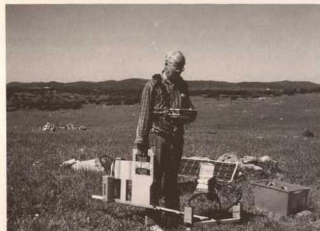
Fig. 2 and 3. Monte da Ponte 1994. Caesium magnetometer Picotesla-system CS2/MEP720 (Scintrex/Picodas) at first application in March 1994
