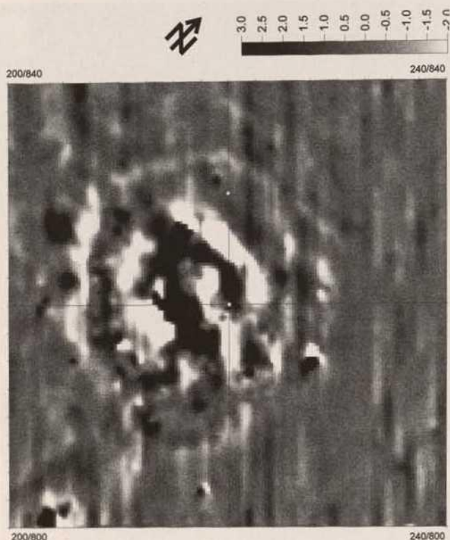
Fig. 4a. Ambrona-Dolmen de la Sima 1998. Magnetogram (detail) of the round barrow with a rectangular chamber. Caesium magnetometry Scintrex SMARTMAG SM4G-Special with duo-sensor configuration, sensitivity 10 pT, raster 0.5/0.25 m, highpass filtering 10 x 10 pixel, dynamics -2.0/+2.0 nT in 256 greyscales, 20 m grid
