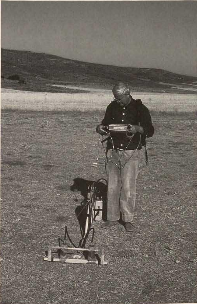
Fig. 1a. Ambrona-La Lampara 1996. Caesium magnetometry using Scintrex SMARTMAG SM4G-Special with duo-sensor configuration
