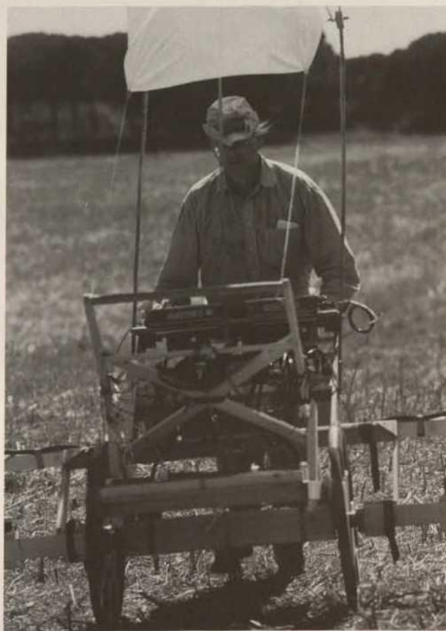
Fig. 1. "Magneto-Scanner" of the Bavarian State Authorities for Monument Conservation at its first test in Ostia Antica 1996, consisting of four caesium magnetometers Scintrex SMARTMAG SM4G-Special with quadro-sensor configuration, two gradiometer consoles-data loggers, power supply (4 batteries 12V/6Ah) and automatic distance trigger mounted on a nonmagnetic chariot, total weight about 50 kg), prototype 1996
