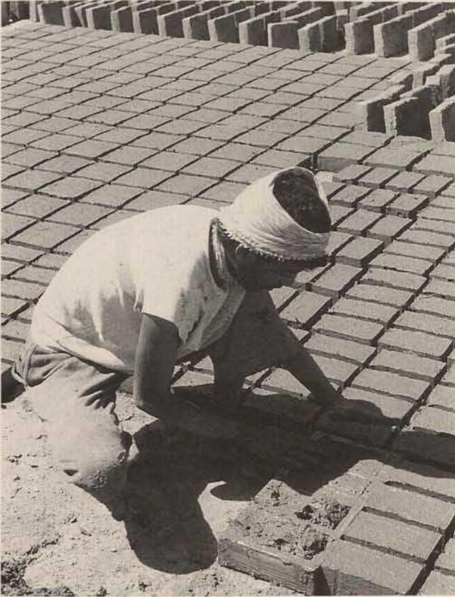
Abb. / Fig. 81. Lehmziegelherstellung in traditioneller Technik, Abstrich und Trocknung / Production of clay bricks according to traditional practice, leveling and off drying
