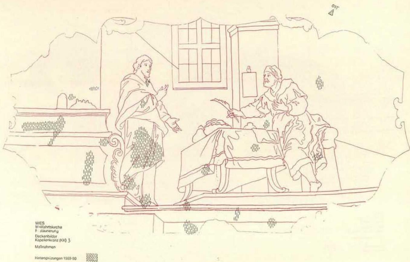
Abb. 50, 51. Dokumentationsfolien «Hinterspritzungen 1989/90» sowie «Kittung» (schwarz) über Schemazeichnung wie Abb. 38 (rot) Fig. 50, 51. Documentation transparencies «showing where injections were made behind the picture» (1989/90) and «where filling compound was applied» (black) over schematic drawing as fig. 38 (red)
