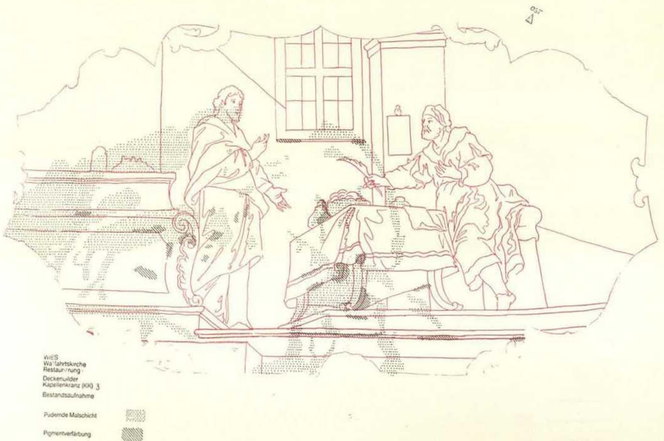
Fig. 46, 47. Documentation transparencies of «smudged areas» and of «powdering paint surfaces and pigment discoloration» (black) over schematic drawing as fig. 38 (red)
