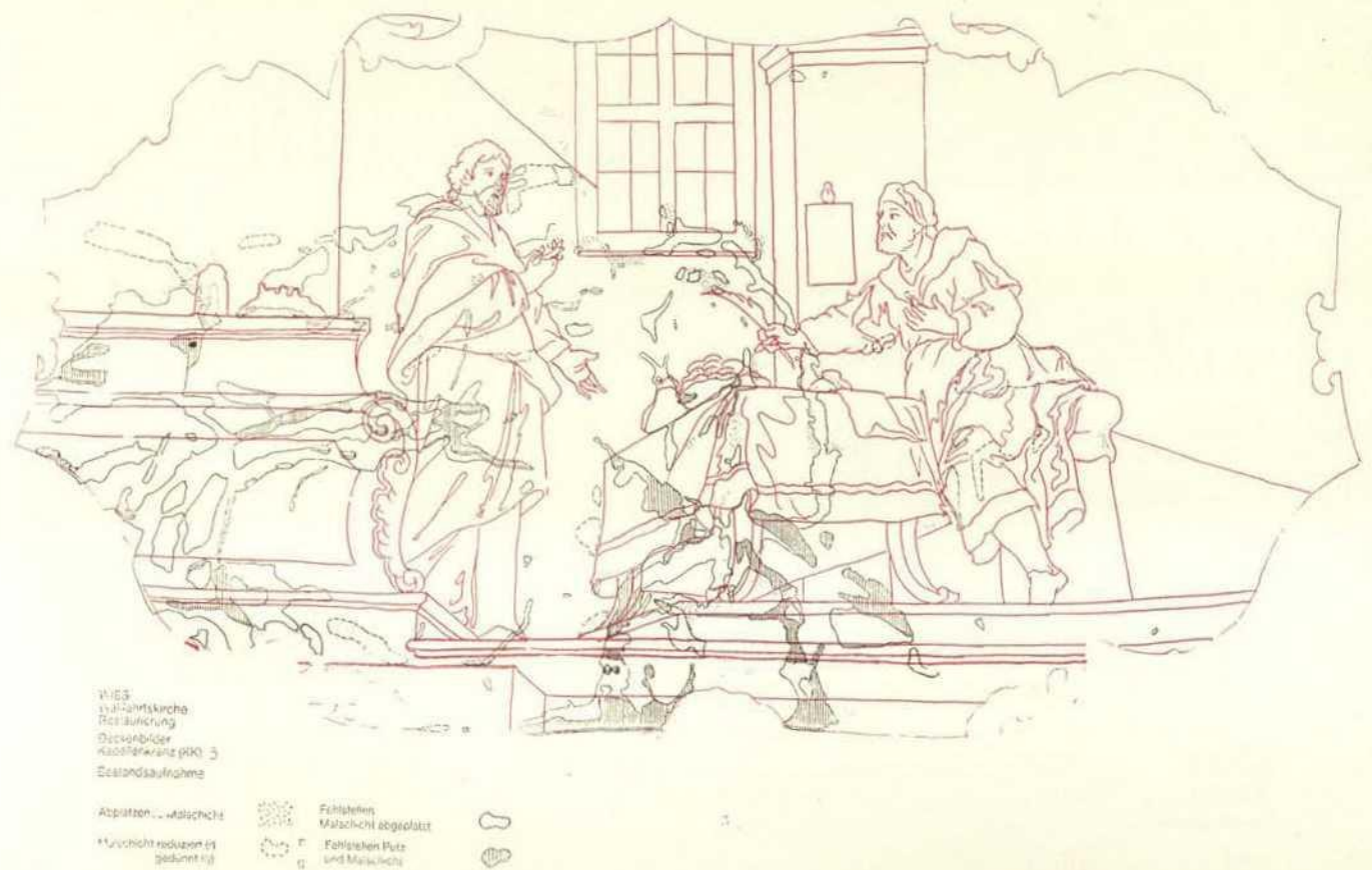
Fig. 42, 43. Documentation transparencies of «cavities» and of «flaking and thinned paint layers, gaps in the paint and the plaster» (black) over schematic drawing as fig. 38 (red)
