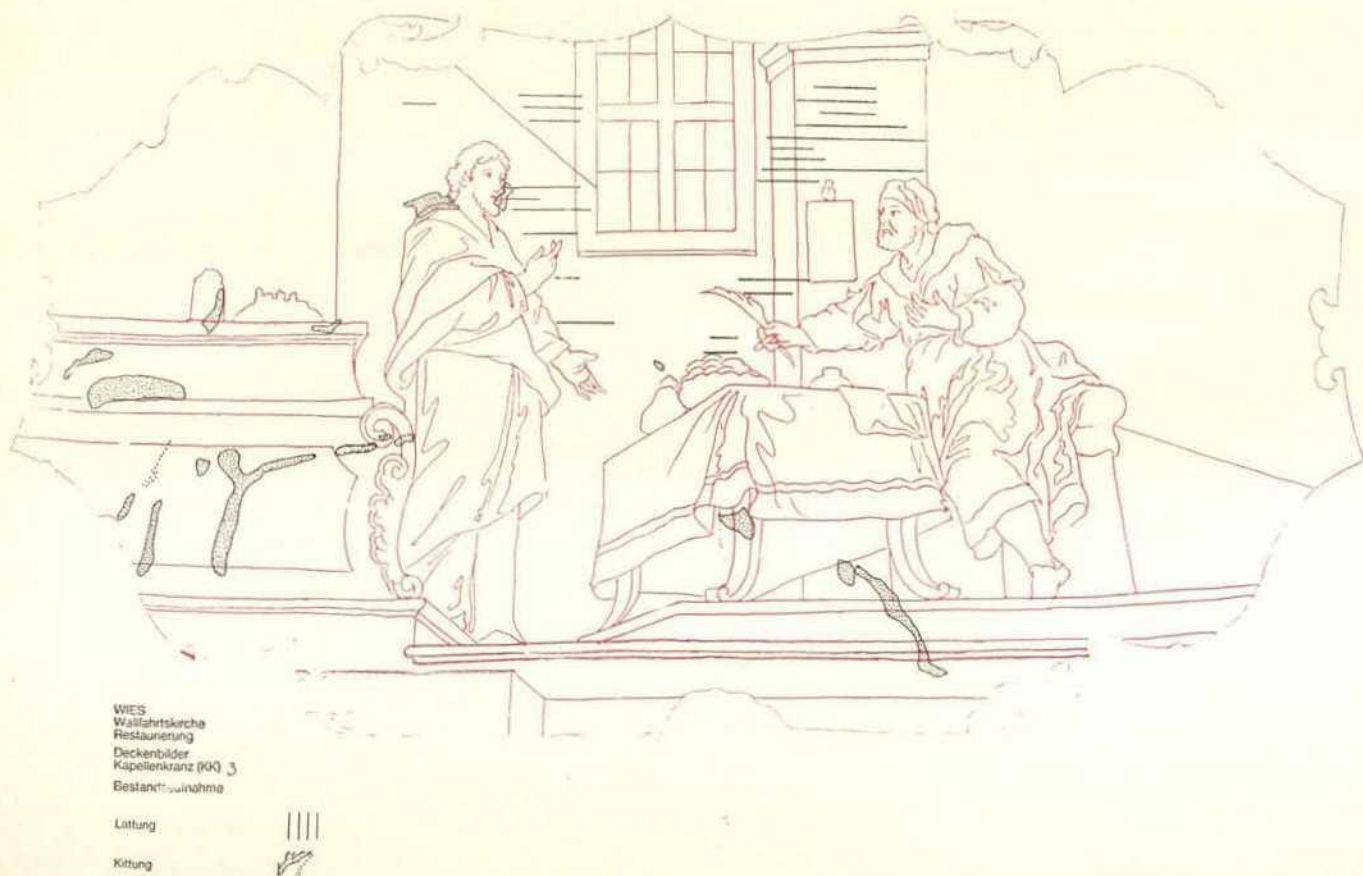
Fig. 40, 41. Documentation transparencies of «separated pieces of plaster, cracks and gaps» and of «lathing and filling» (black) over the same schematic drawing as fig. 38 (red)
