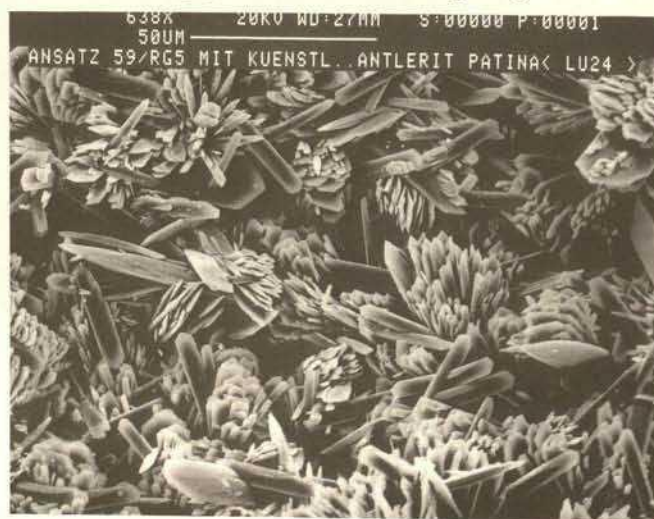
Fig. 7. SEM micrograph: artificial antlerite on Rg5 alloy
