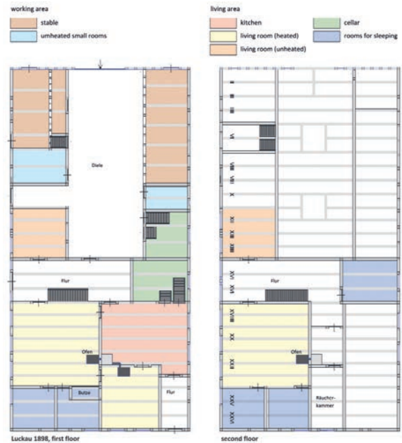
Fig. 14 Ground plans of the first and second floors from one of the last hall houses built in the Wendland
