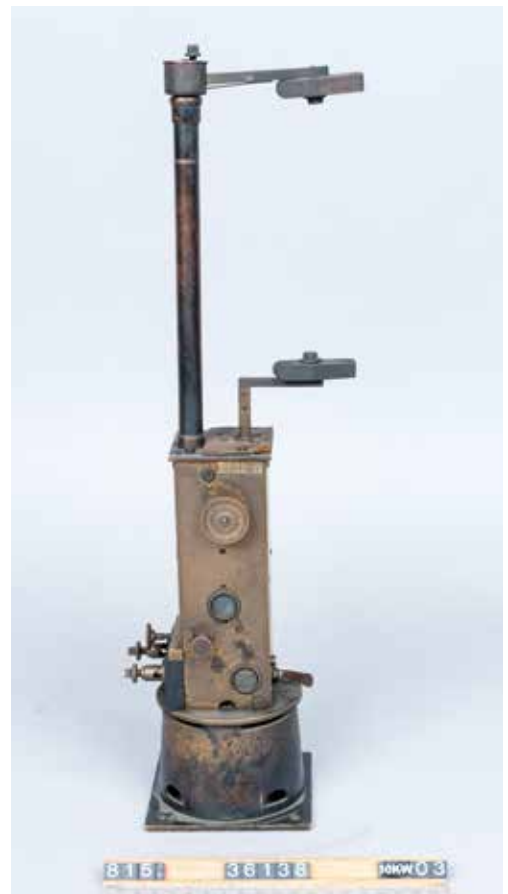
Abb. 6: Bogenlampe, Siemens & Halske, System Hefner-Alteneck (Inv.-Nr. 36138)
