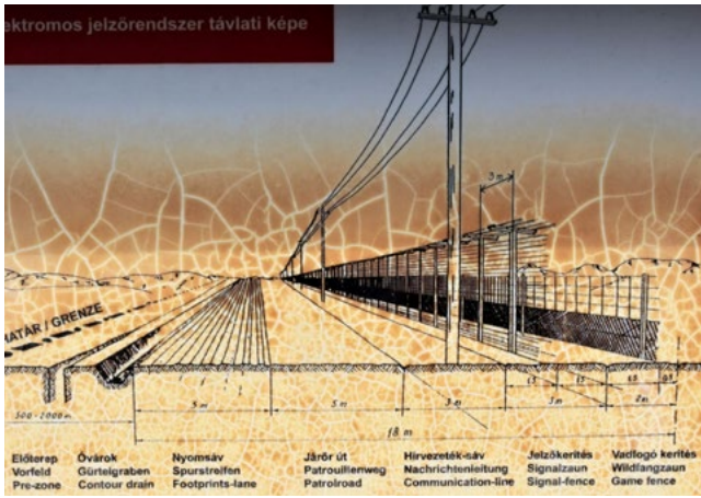
Fig. 3: Typical section of the border installation (photo taken at the pan-European picnic memorial)
