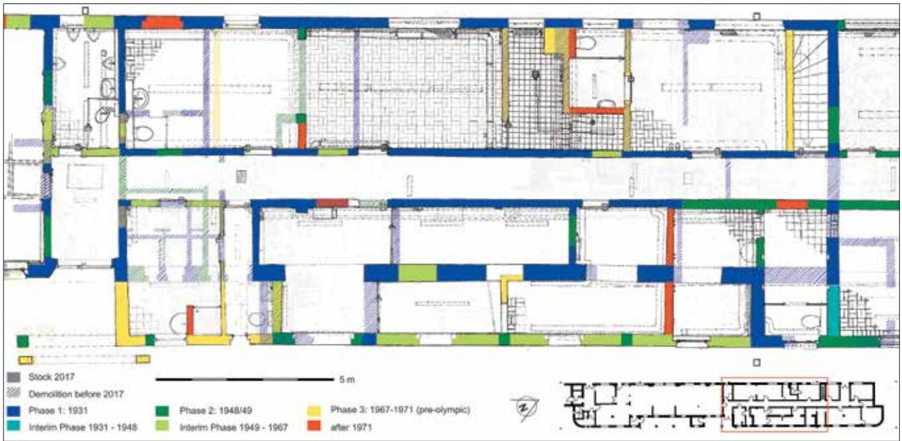
Fig. 2 xtract of the true-to-deformation measurement, showing the construction phases
