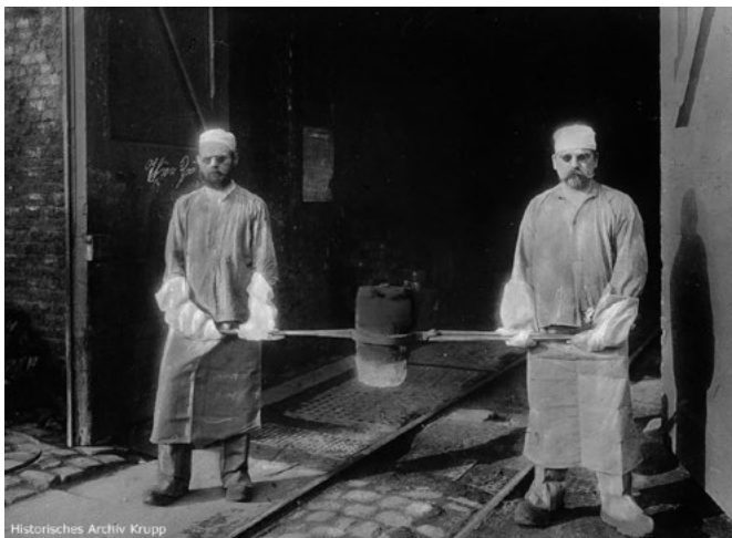
2 Crucible carriers at Krupp steel-works, from the series «Krupp Eisen und Stahl», c. 1903, colored photograph, Essen, Historisches Archiv Krupp
