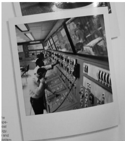
4 John Hill, This 60-foot console monitors each step of the coating process [...] concave viewing mirrors coated with high-reflectance aluminium , Fotografien, in: Polaroid Corporation Annual Report for 1973 , hg. v. Polaroid Corporation, Cambridge/Massachusetts 1974
