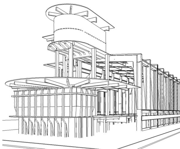
Fig. 4: The reinforced-concrete framework of the power station building. CAD simulation (StroyNauka, Minsk)
