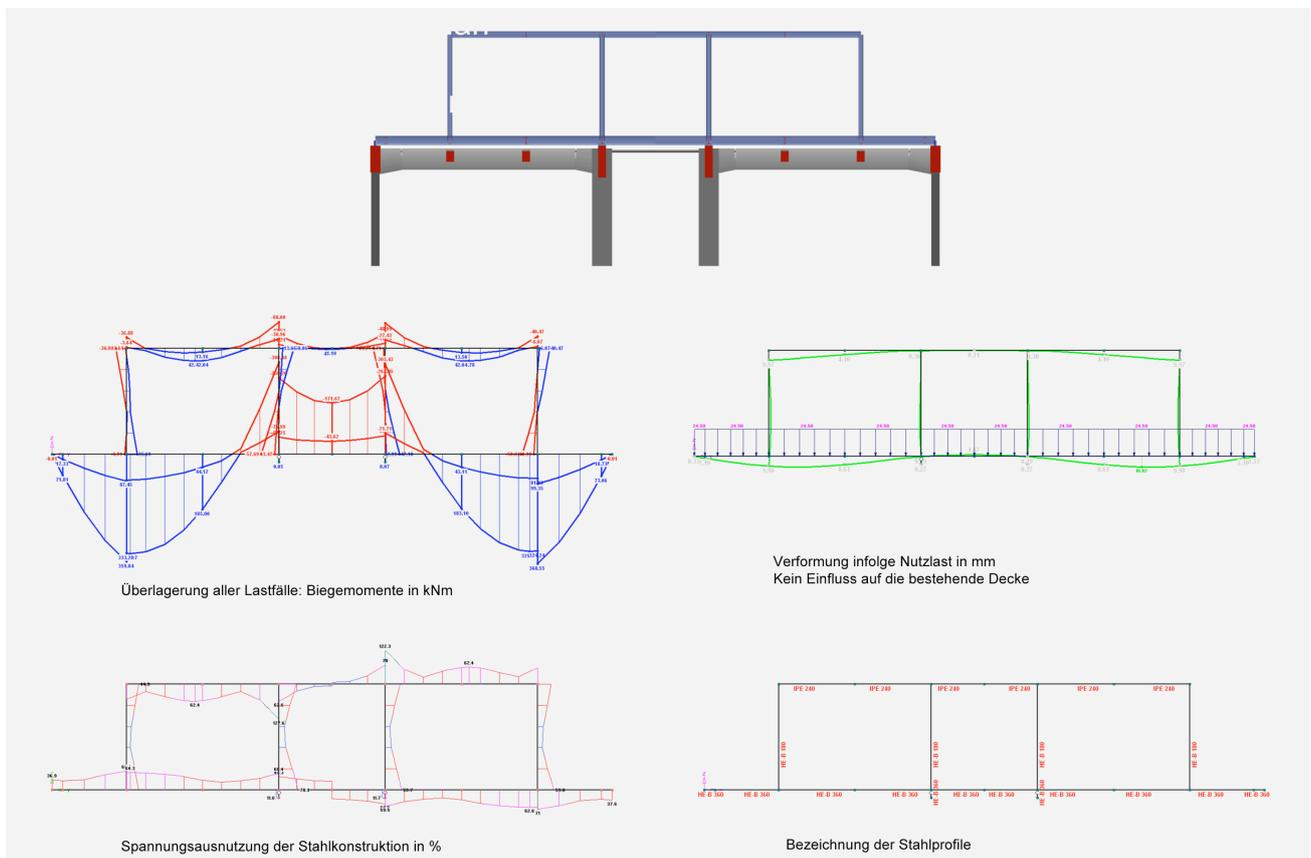
were used to determine the level of stress from snow and wind. Light-weight steel structures with glass sheeting were selected provisionally as new architectural elements – metal-rod superstructures over the former dyeing sections. If the superstructures are built with light-weight membrane sheeting for lighting, this approach is also fully feasible. The amount of the wind pressure would be identical in both cases (fig. 34).
