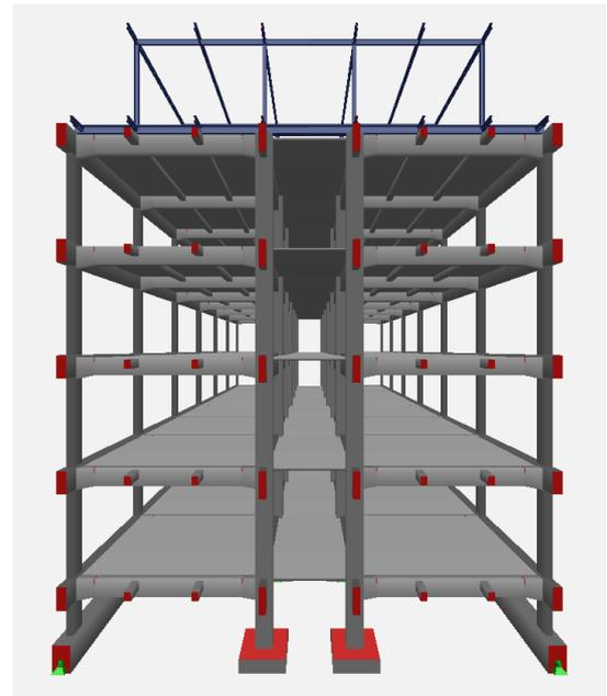
Fig. 38: Assessment of a new penthouse on the framework structure on a main fabric building (the Office of Professor Pfeifer and Partners, 2008)
