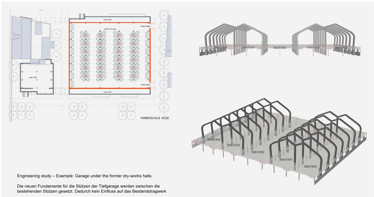
Fig. 35: The possibility of expanding the original frame structure of the dyeing workshop through an underground garage (the Office of Professor Pfeifer and Partners, 2008)
