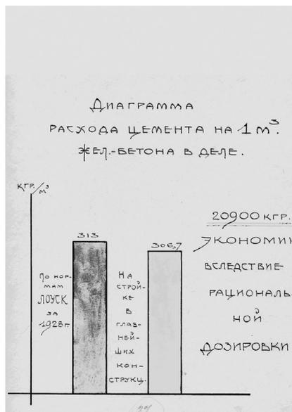
Fig. 8 (a, b): Diagrams illustrating the strength of the concrete and the amount of cement used in the concrete, 1928–1929
