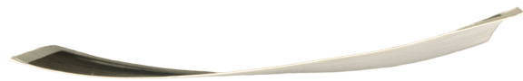
Fig. 2: Graphics atlas, Fiber-based paper supports look and feel like paper on the back. Prints with a heavy weight paper may tend to curl slightly (Image of a photographic object) Digital image, undated.
