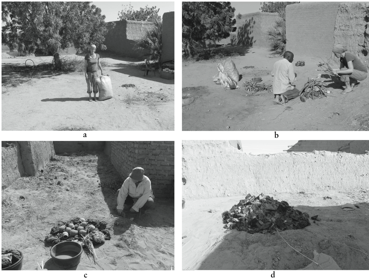
Fig. 3: Experimental firing. a = supplying fuel; b = preparing the bonfire; c = positioning the thermocouple; d = firing; b = acacia wood used as fuel, c – d = cow dung used as fuel (photos a – b: M. Daszkiewicz, c – d: M. Wetendorf).
