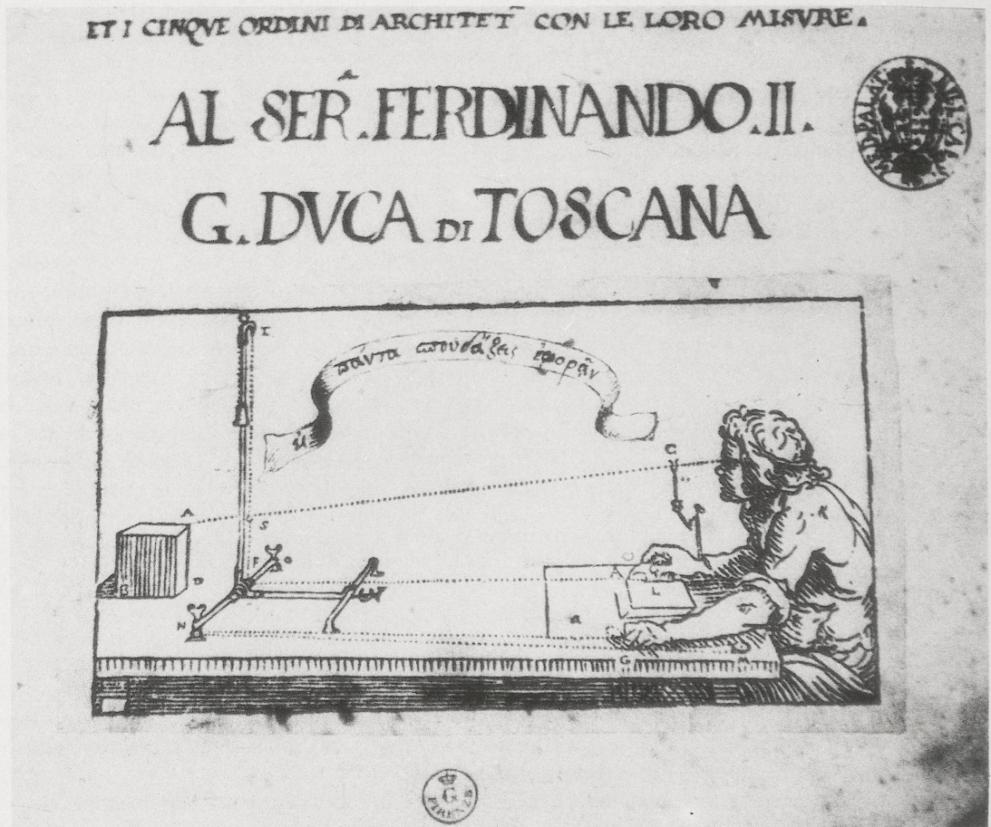
4 Draftsman using Cigoli’s perspectograph to draw a cube in perspective, from Lodovico Cigoli, Prospettiva pratica , title-page.
