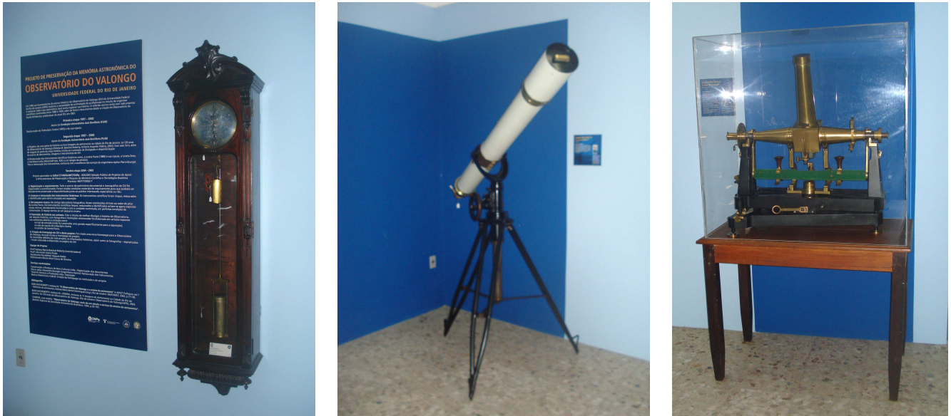
Figure 13.7: Some of the instruments in the Observatório do Valongo collection (from left to right): a pendulum clock, a refractor (Zeiss) and a meridian refractor (Julius Wanschaff) (MAST archives)
