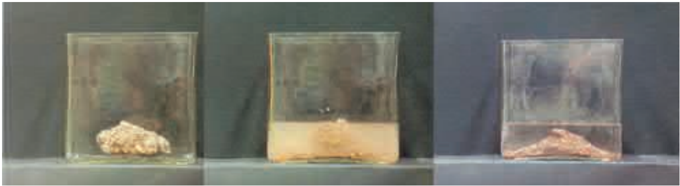
Fig. 3. Testing the conglomerate: dry specimen (left), after a few seconds under water (centre), after sedimentation (right)
