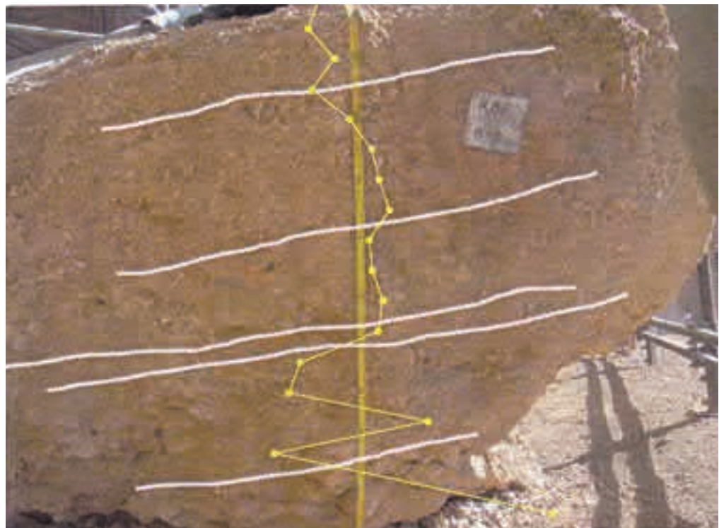
Fig. 5. Fragment KBF_015 from within the niche. White lines approximate prominent lithological layers, yellow curve displays magnetic susceptibility k_{in} 10–5 SI Units. Vertical dimension of the fragment is 1.2 meters.
