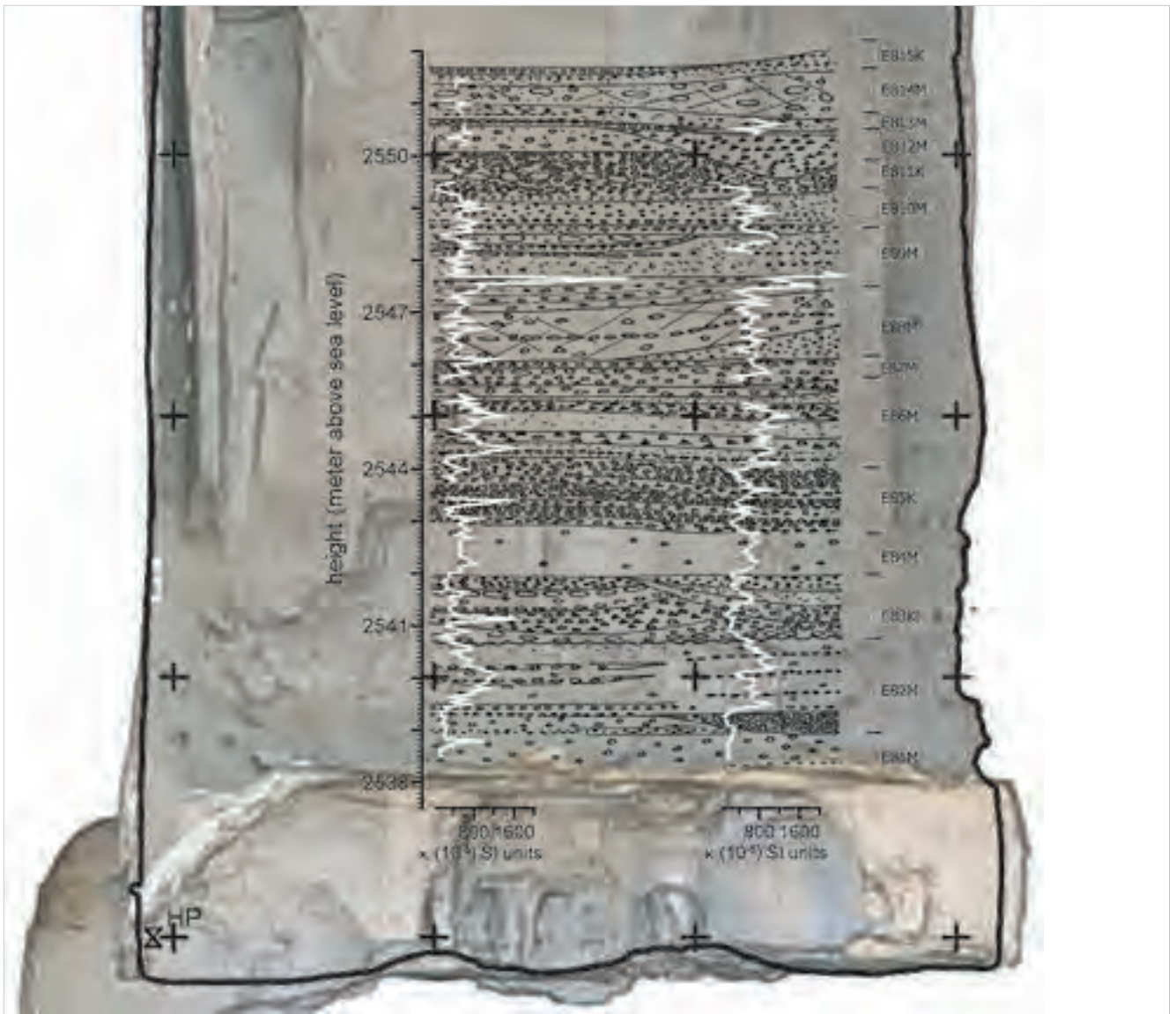
Fig. 4. Schematic of the eastern Buddha niche lithology indicating the results of the two magnetic susceptibility profiles. Major lithological units shown in more detail in figure 3. Height is in meters above sea level, profiles start at 2538.4 m.a.s.l. levelled from the reference point BP1 at 2535 m.a.s.l. Background 3D scan is courtesy of RWTH Aachen group.
