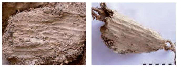
Fig. 20. Traces of fingers in the undercoat layers: Left: Fragment on-site. Right: Fold ridge of Western Buddha, fragment GBL 1088: Undercoat of a fold ridge of the Western Buddha [Melzl]
