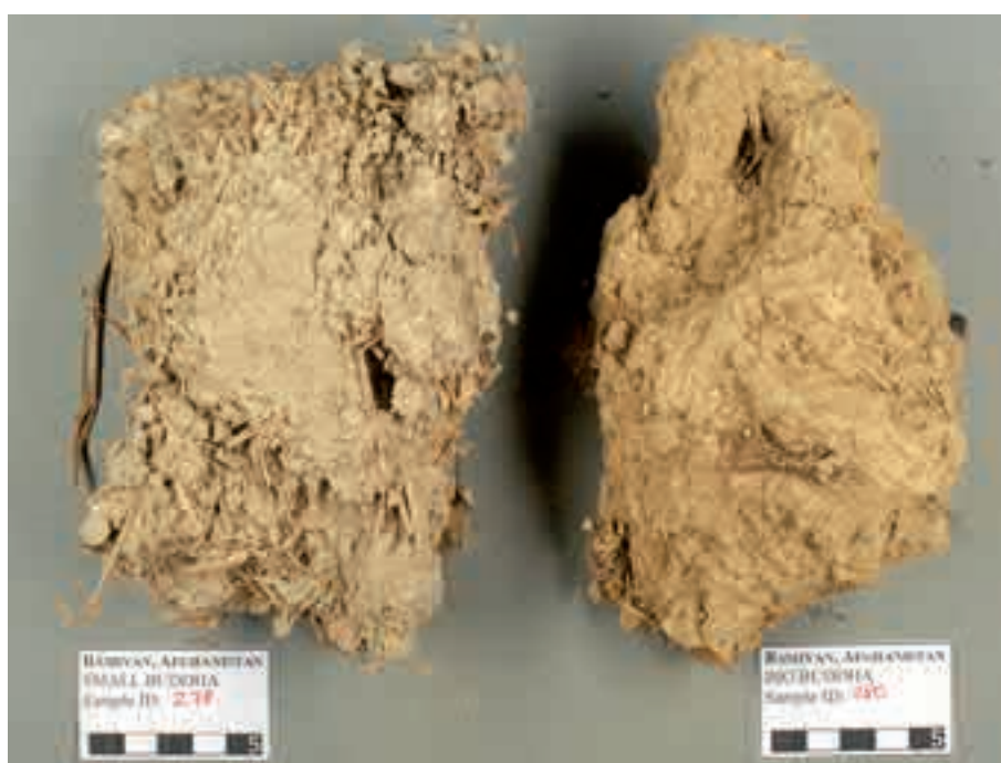
Fig. 1. Loam plaster fragments of the Eastern Buddha (sample 278, left) and the Western Buddha (sample 280, right) [Höfle, Thiemann]
