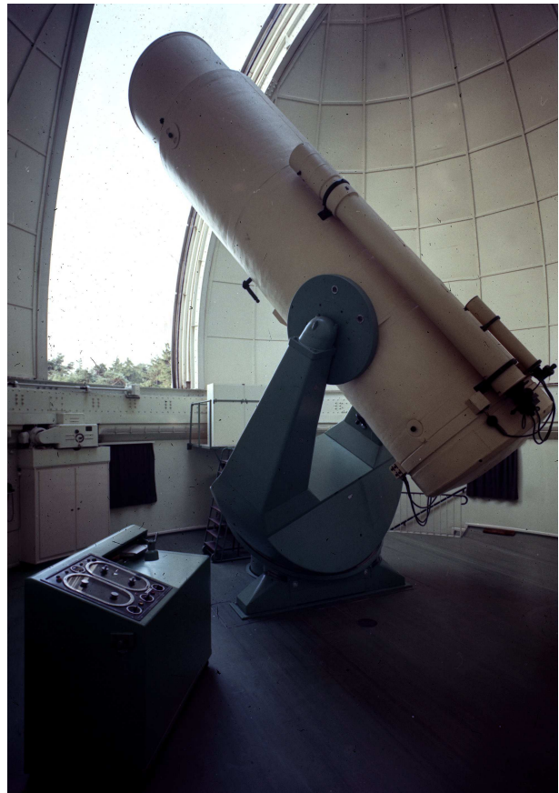
Figure 5.19: Large 80 cm Hamburg Schmidt telescope, Zeiss, Jena, Heidenreich & Harbeck, Hamburg, 1954 (Hamburg Observatory)
