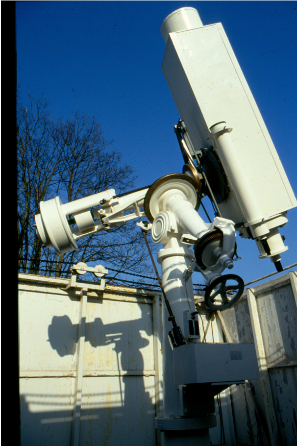
Figure 31.9: 40 cm Salvador reflector (1967) and 23 cm zone astrograph, Zeiss, Oberkochen (1973) (Hamburg Observatory)
