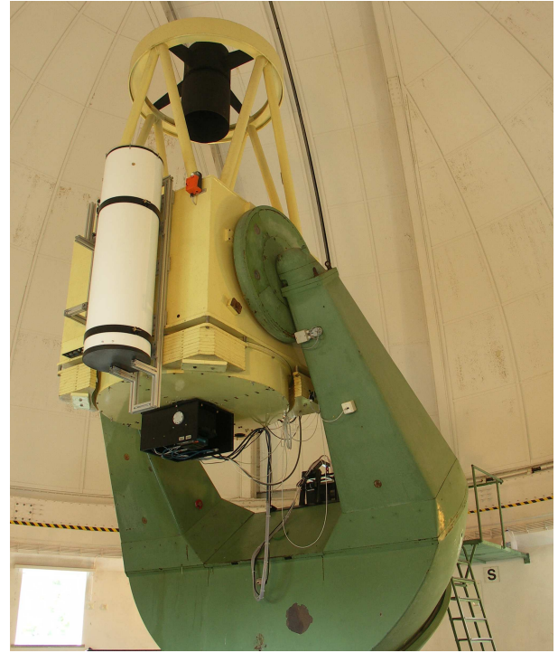
Figure 31.7: Large 80 cm Hamburg Schmidt telescope, Zeiss, Jena, Heidenreich & Harbeck, Hamburg, 1954; 1.20 m Oskar-Lühning telescope, Grubb, Parsons & Company, 1975 (Left: Hamburg Observatory, Right: Photo: Matthias Hünsch)
