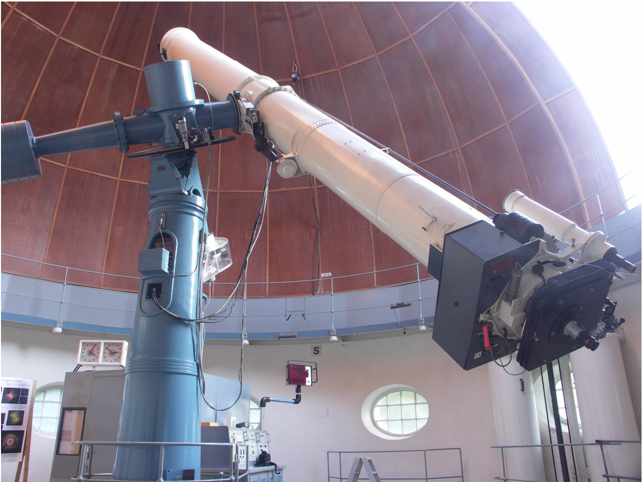
Figure 31.4: Large refractor (60 cm, 9 m), Mechanics: A. Repsold & Söhne, Hamburg, 1911, Optics: Steinheil, Munich (visual objective, 1914, photographic objective, 1925) (Photo: Matthias Hünsch)
