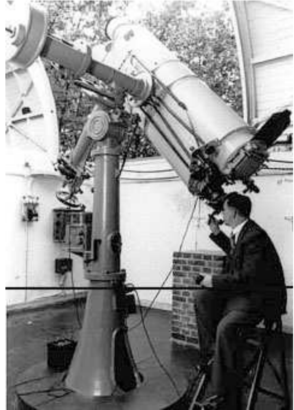
Figure 31.5: 34 cm Lippert astrograph in its original configuration, Carl Zeiss, Jena, 1911; AG Astrograph, Carl Zeiss Jena, 1924 (Hamburg Observatory)
