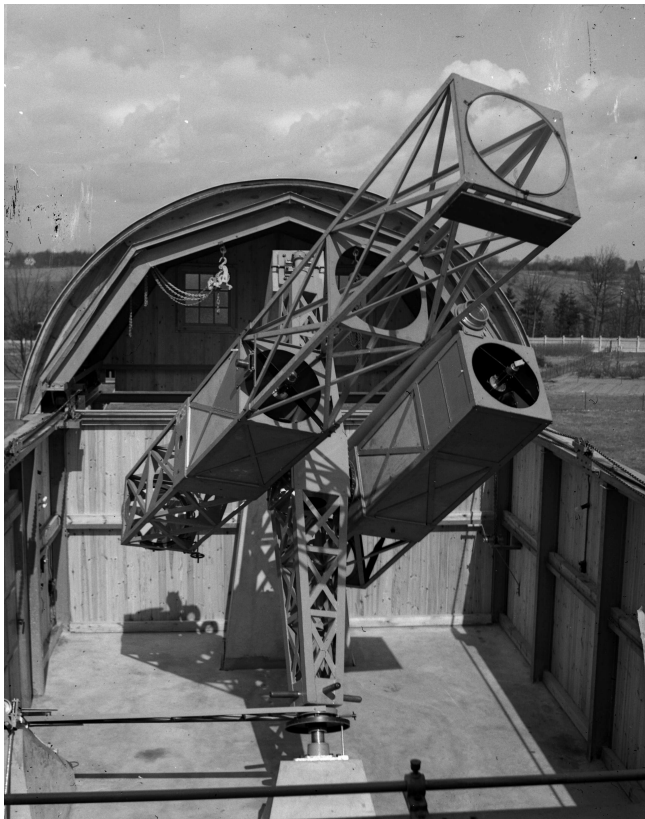
Figure 31.8: 60 cm double reflector, Bernhard Schmidt, Hamburg, 1934: 60 cm Schmidt telescope and 60 cm Newtonian-type (Hamburg Observatory)
