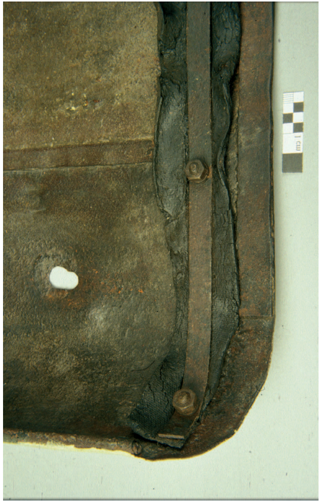
Figure 32.7: Detail of large device with corroded metal, dirt and degraded rubber, material before conservation; Detail as in the left figure, after cleaning, consolidation and conservation of the materials (HTW, Halm)
