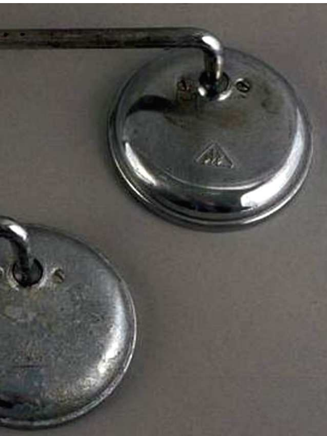
Figure 32.4: Missing areas of chrome on the back of a car mirror; Metal leaf in a galvanic bath: chrome is being plated; As above, after filling missing area with the plated metal and gilding oil; N. B. for New Built on the head of a reconstructed screw to replace a missing one (HTW, Grundmann, Matin Pour, Grundmann, Gehrman)
