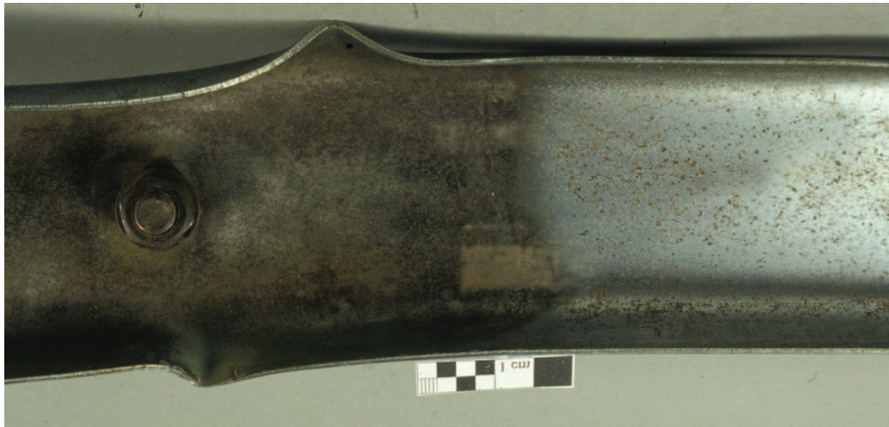
Figure 32.6: Dirt and corrosion underneath a van, 1950; Underneath the historic van after cleaning and conservation; Chrome plated steel covered by corrosion products; before (left) and after (right) the local cleaning by scalpel (HTW Berlin; HTW, Grundmann)
