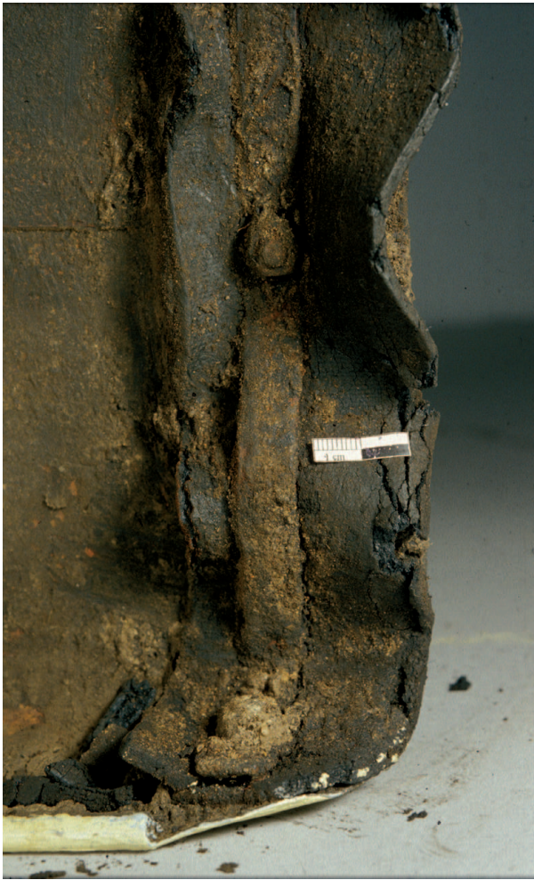
Figure 32.7: Detail of large device with corroded metal, dirt and degraded rubber, material before conservation; Detail as in the left figure, after cleaning, consolidation and conservation of the materials (HTW, Halm)
