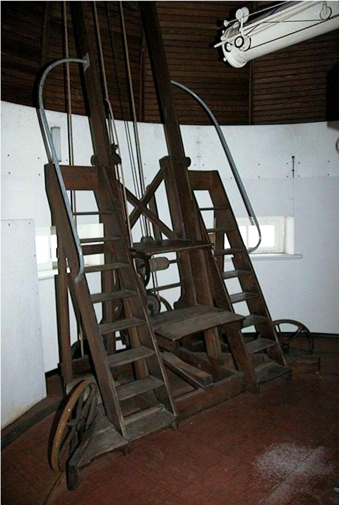
**Figure 38.1:** *Observing chair of the Equatorial Telescope (Hamburg Observatory)*
