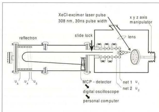
Fig. 5. Section of the laser desorption mass spectrometer.
