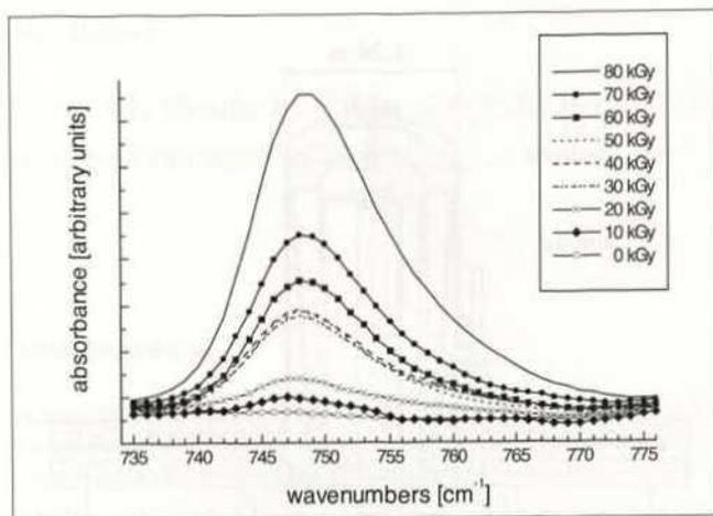
Fig. 2. Electron beam curing of Plex 6803-1 at different doses (one step treatment).
