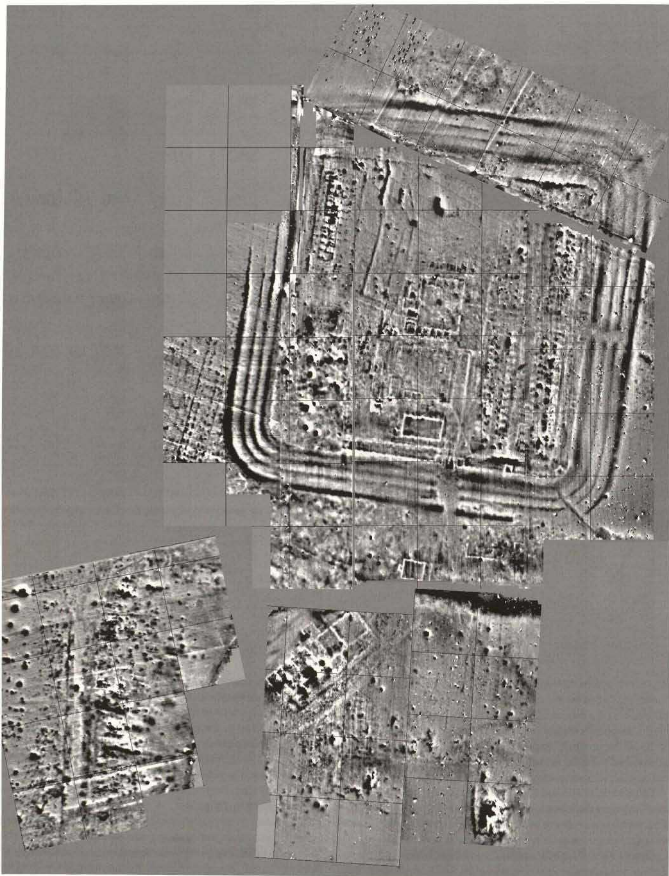
Fig. 7. Roman castellum at Ruffenhofen. Magnetogram of the castellum with the vicus and the baths. SMARTMAG SM4G-Special as quadrosensor. Sensitivity 0.01 nT (10 picotesla), raster 0.1/0.5 m interpolated to 0.25/0.25 m, dynamics -7.0/+7.0 nT in 256 gray scales (black/white), 40 m grid, magnetometer prospecting H. Becker, Mag.Nr. 6928/074-00A.
