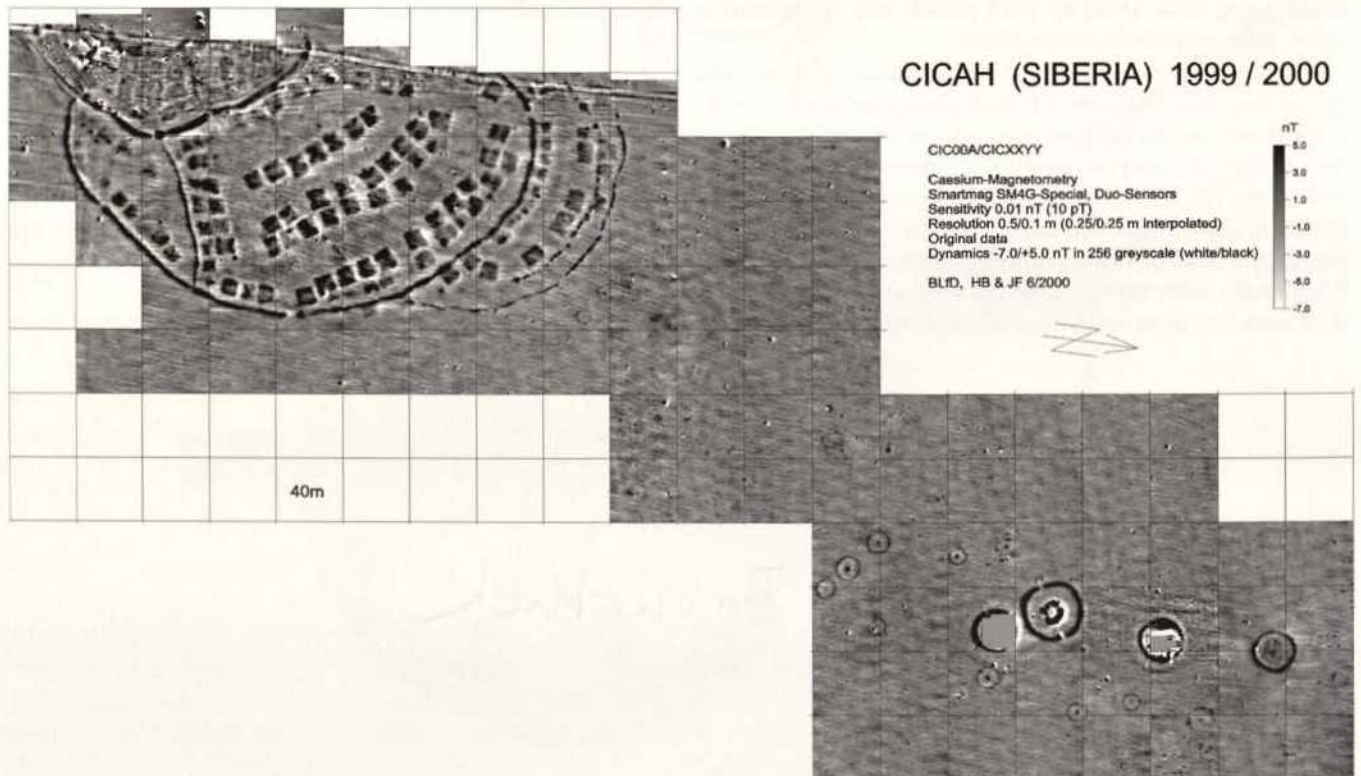
Fig. 2. CicaH (Siberia). Magnetogram of the measurements from 1999-2000 with the entire Scythian settlement (city) from the 8 th -7 th centuries BC and the (presumably later) necropolis with four large kurgans . SMARTMAG SM4G-Special as duo-sensor. Sensitivity 0.01 nT (10 picotesla), raster 0.1/0.5 m interpolated to 0.25/0.25 m, dynamics -5.0/+5.0 nT in 256 gray scales (black/white), 40 m grid, magnetometer prospecting H. Becker und J. Faßbinder.
