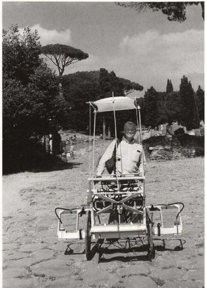
Fig. 5. Ostia Antica 1996. "Magnetoscanner" on its first run, magnetic prospecting with two SMARTMAG SM4G-Special in quadro-sensor configuration on a non magnetic cart (total weight = 48 kg)
