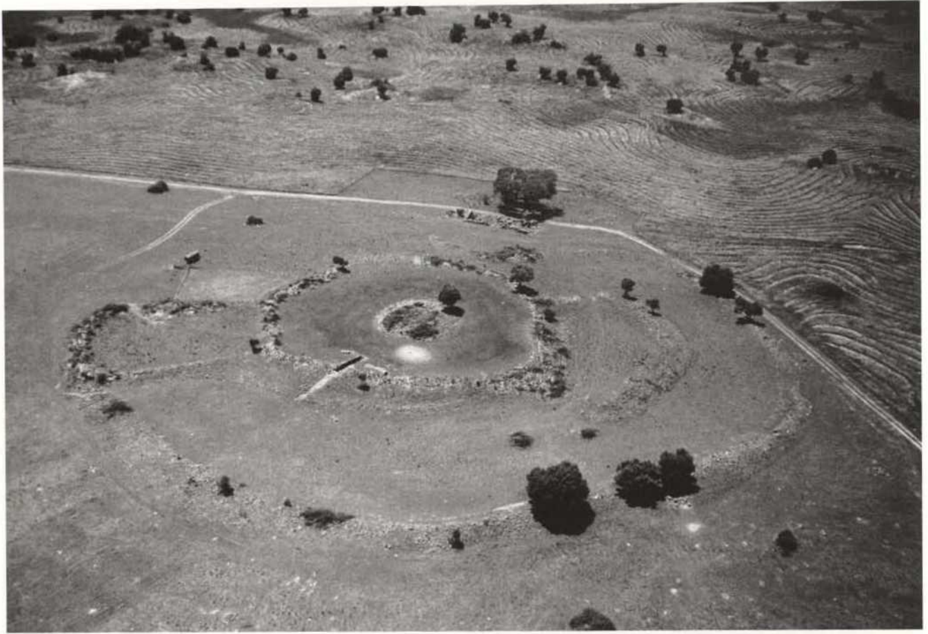
Fig. 6. Monte da Ponte 1997. Aerial view of the Copper Age fortified settlement with signaled control points (20 m grid) on the ground by Ruprecht and Michaela Steinman as base for an photogrammetric evaluation for a plan of all stones
