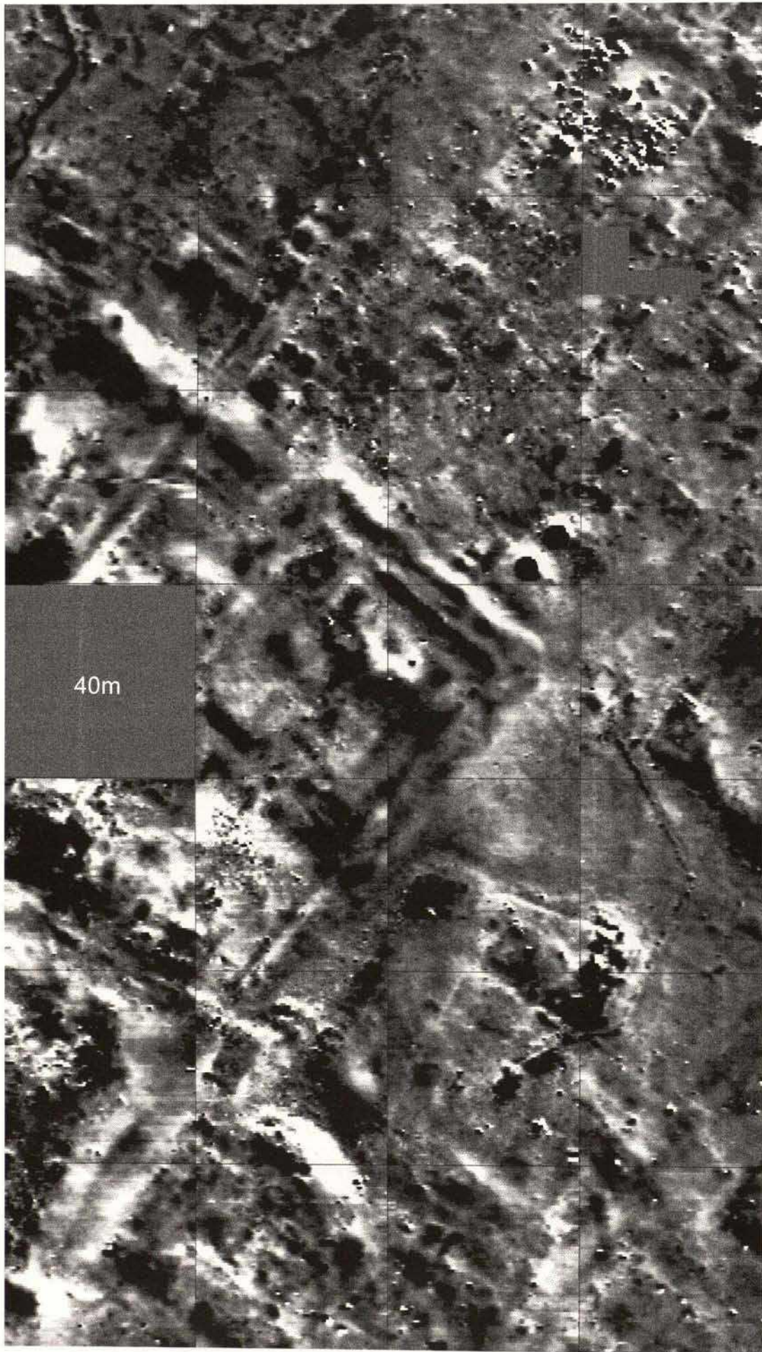
Fig. 1. Rusafat-Hisam 1997/98, palace complex III/IV. Magnetogram as digital image, caesium magnetometer Scintrex SMART-MAG SM4G-Special with duo-sensor configuration, sensitivity 0.01 nT, raster 0.5/0.25 m after resampling, reduction to the line-mean, dynamics -3.2/+3.2 nT in 256 gray-scale (white/black), 40 m grid
