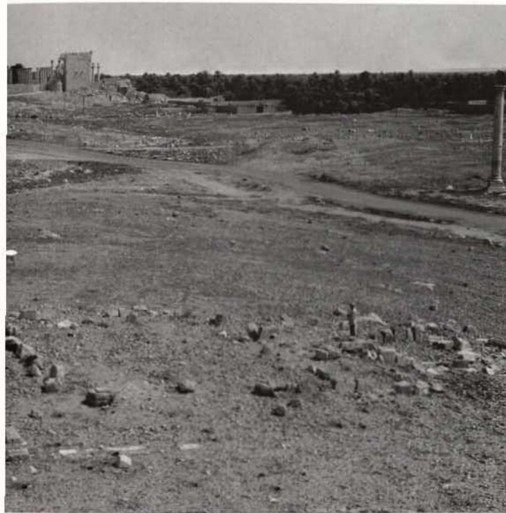
Fig. 1. Palmyra 1997. Western corner of the Hellenistic city situated between the wadi, Roman city wall and the oasis to the south, the huge building complex in the upper part in the middle is the temple of Bel. Extrem oblique view from a hydraulic crane from 8 m high; marked control points on the ground (white)
