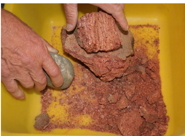
Figure 3. A naturally eroded granite stone collected from the coast was easily crushed by hammering it with another stone (photograph by the author).
