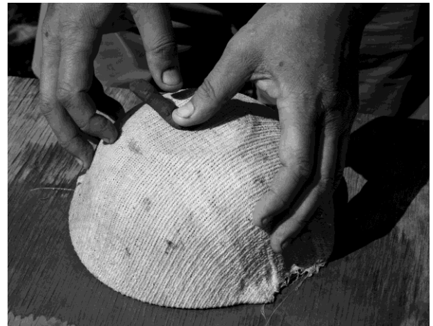
Fig. 3. A convex hemispherical solid mould covered with fabric and used for construction of experimental vessels.
