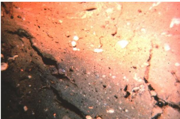
Figure 9. Section across a tuyere from the Bronze Age smelting site at Timna, Israel, with just a little quartz temper (cf. Figure 3; M.S. Tite / British Museum).
