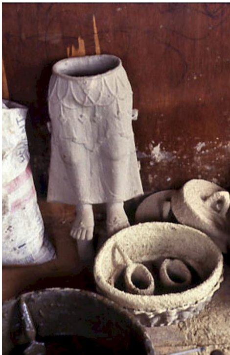
Figure 13. The wax model of the lower part of a statuette with the first coating of fine clay in place. Patan, Nepal, 1987 (P.T. Craddock).
