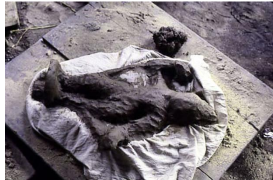
Figure 14. Mould for casting a figure, with the outer layer of coarse clay in place. Swamimalli, Tamil Nadu, 1986 (P.T. Craddock).
