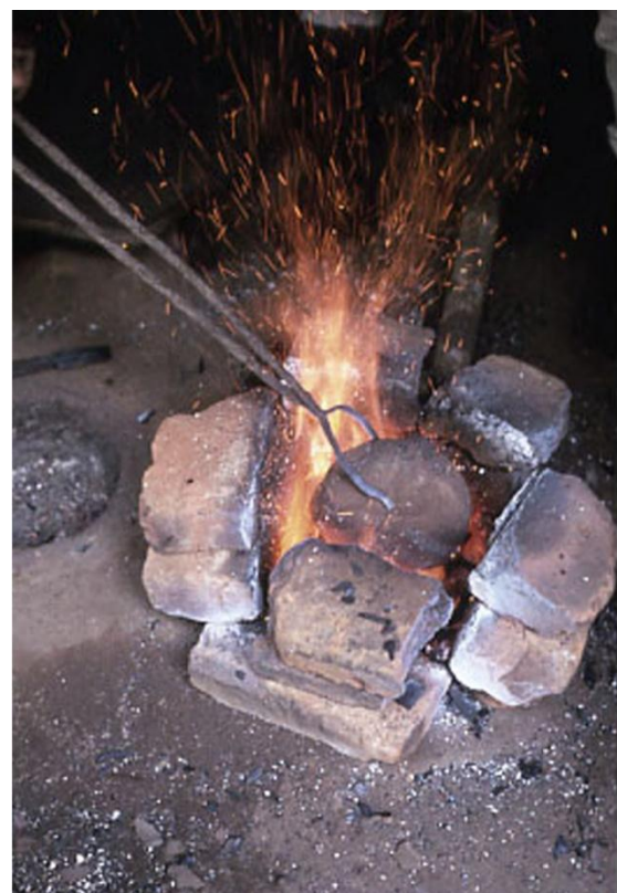
Figure 3. Removing the mould and crucible from the hearth after firing with the crucible beneath, after a short period to cool slightly the unit will be inverted allowing the molten bronze to flow down into the mould (P.T. Craddock).
