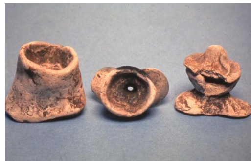
Figure 15. A selection of Romano-British sprue cups, which held a reserve of molten metal above the mould as the metal cooled and contracted (British Museum copyright).
