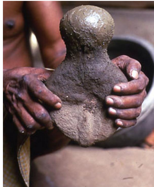
Figure 2. The finished mould and crucible firmly luted together with clay heavily tempered with rice husks, ready for firing (P.T. Craddock).
