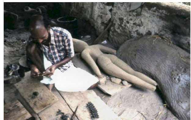
Figure 18. Large core for the direct lost wax casting of a life-size figure. Note a completed mould to the right. Swamimalli, Tamil Nadu, 1986 (P.T. Craddock).
