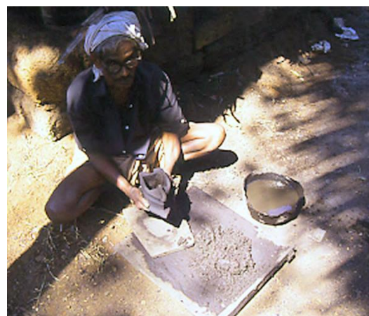
Figure 12. Application of fine clay to the wax of what will be a brass smoothing iron. Kodumunda, Pattambi, in Kerala, 1994 (P.T. Craddock).
