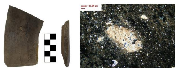
Figure 3. Sample no. IAIII-4 is a thin dark grey ceramic (left), and a dark red rim around a calcite grain illustrates the concentration of iron oxide (right).
