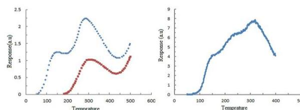
Figure 3. Thermoluminescence glow curves of a ceramic containing calcareous microfossils give a date of  $1817 \pm 84$  BP.
