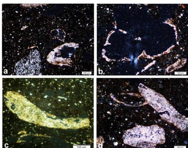
Figure 6. *Qizlar Qal'eh*: micrographs of thin section ceramic samples showing: (a) *Dicarinella* sp.? (b) *Dicarinella* sp.; (c) Ostracod and large massive bioclast; (d) Ostracod and undetermined bioclast (brachiopods?, echinoderms?).
