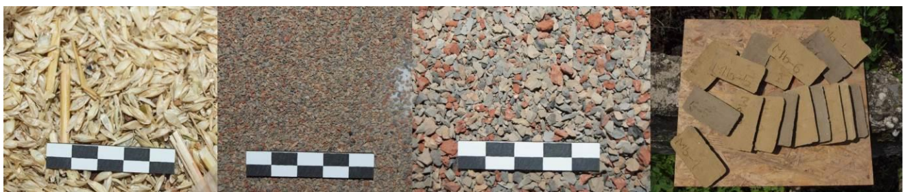
Figure 5. Temper used in the briquettes showing chaff with straw and grog grains in two sizes (photographs by A. Kudelić).
