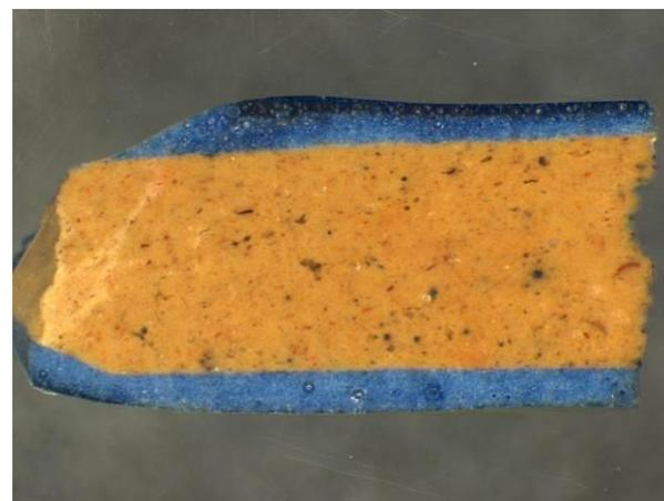
Figure 2a. Optical microscopy of the polished maiolica sample in the resin block.
