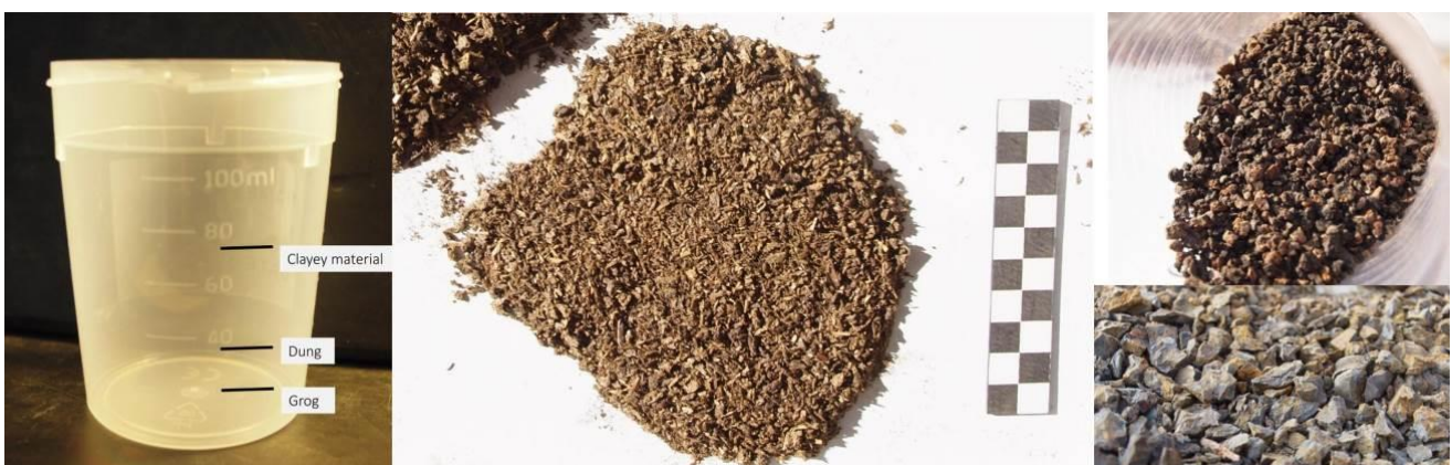
Figure 6. Cup with volume markings of clay and temper used in the experiments with cow dung, grog and clay pellets (photographs by A. Kudelić).
