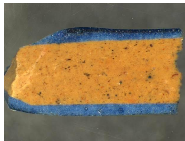
Figure 2a. Optical microscopy of the polished maiolica sample in the resin block.
