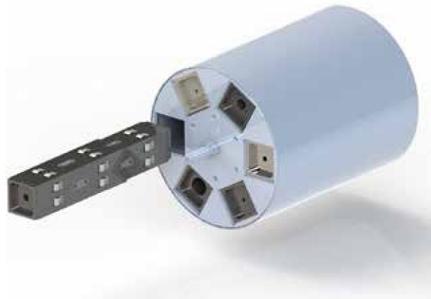
Fig. 3 The rotary drum containing six different collimators with pinhole diameters from 2 mm to 71 mm. The collimators have a length of 800 mm, which effectively stop fast neutron and gamma background and are fabricated from borated steel to minimize activation through neutron capture. – (TU München – FRM II).
