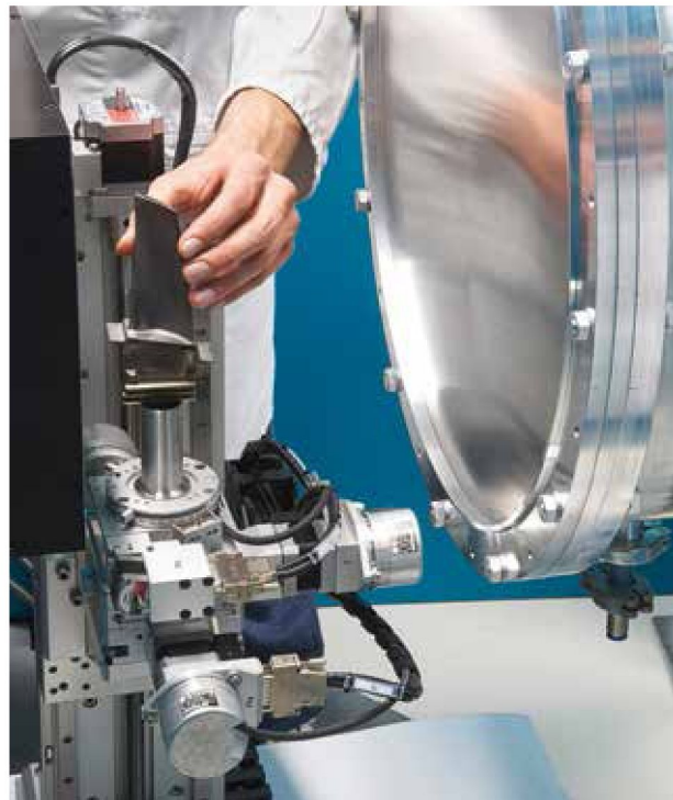
Fig. 4 The sample position in experimental chamber 1. The sample can be accurately positioned in the horizontal and vertical direction in front of the detector. Furthermore, a rotary stage is available for tomography, which is mounted on two goniometers for exact alignment of the rotation axis with respect to the detector. – (TU München – FRM II).
