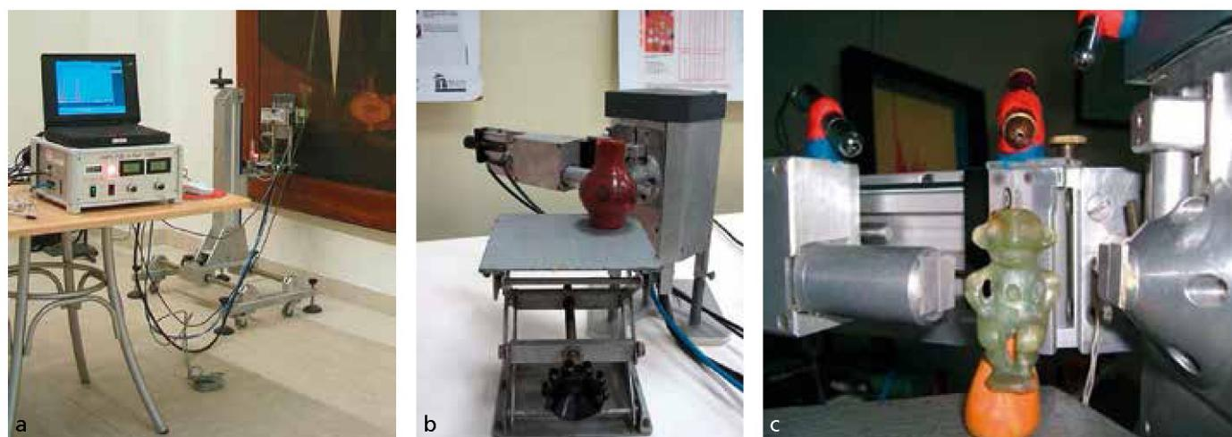
**Fig. 1** Portable X-ray system: **a** full setup. – **b** measurement head during XRF analysis. – **c** XRD analysis. – (K. J. Carlson).
