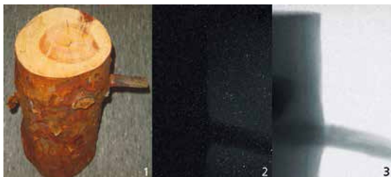
Fig. 1 Piece of log (1) with the unprocessed neutron radiograph (2) affected with spotted flaws and after appropriate image processing (3). – (Photo, X-ray and image processing K. Osterloh).
