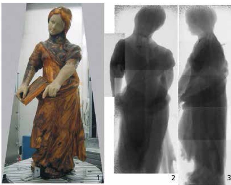
Fig. 4 Sculpture »Virtue of Hope« (1) with neutron radiographs in frontal (view from behind) (2) and lateral direction of penetration (3). – (Photo and composed neutron radiographic image by the authors).
