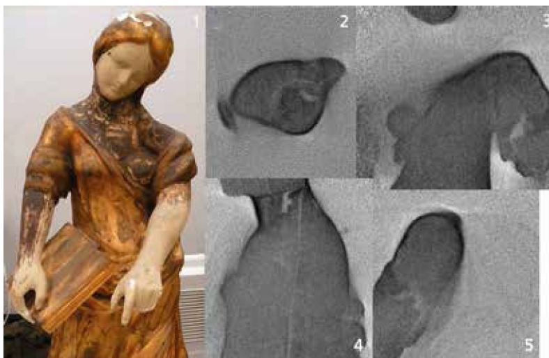
Fig. 5 Neutron CT of the sculpture »Virtue of Hope« (1) with a cross section in the lower neck region (2) and longitudinal sections in different directions (3-4). The region in the upper left arm (5) shows indications of repair (frontal in the upper right panel and saggital in the lower right one) matching with the relative spotless appearance in the photograph (left). – (Photo and processed neutron CT images by the authors).
