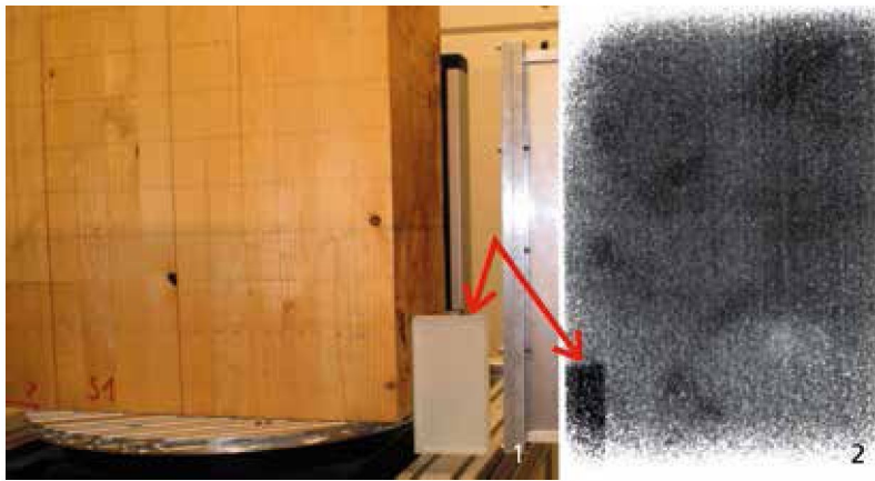
Fig. 3 1 penetration of fast neutrons through a layer of 50cm wood. – 2 beam direction from left to right, radiographic image showing the shade of the Perplex block at the bottom (red arrows), filtered radiographic image showing several internal knots more clearly. – (Photo and processed neutron radiographic image K. Osterloh).
