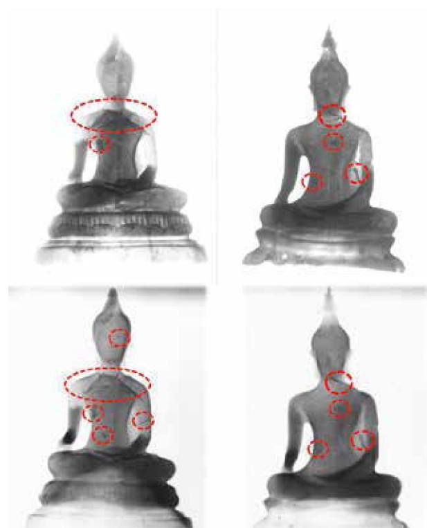
Fig. 3 Comparison of XR and NI greyscale images of two Buddha sculptures (S1 and S2). – (© by the authors).
