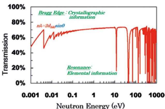
Fig. 1 Example of a transmission spectrum indicating the Bragg edges at low energy regions and resonance peaks at higher energy.
