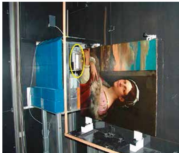
Fig. 1 Irradiation chamber of instrument B8. The yellow ellipse marks the end of the neutron guide. The painting is mounted under a small angle with respect to the neutron guide and is moved up and down in order to provide a homogenous irradiation over the whole surface.
